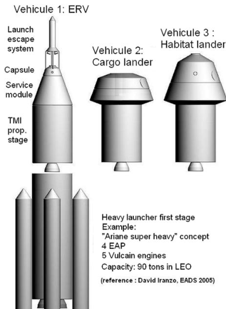
**Figure 7:** Heavy launcher, TMI propulsion stage and three types of vehicles.
