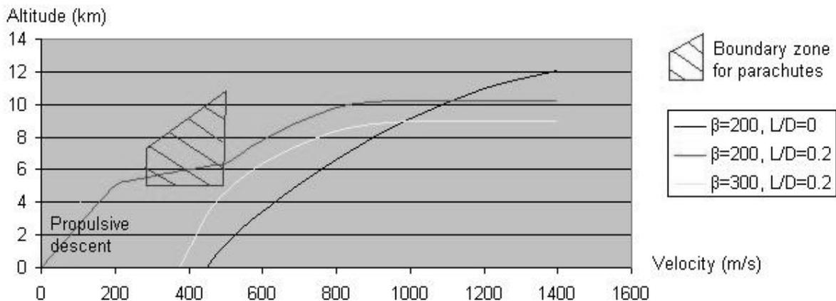
**Figure 1:** Descent configurations according to different ballistic coefficients and L/D values.
