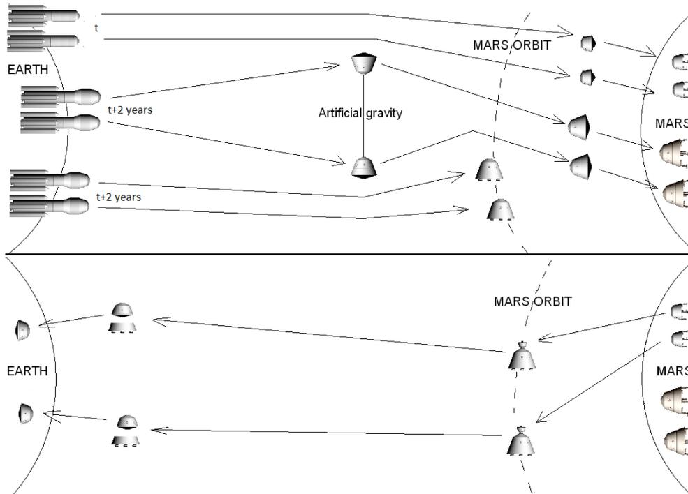
**Figure 2:** Standard option. There are six launches. Two cargo vehicles and two habitat vehicles are sent to the surface of Mars while two ERV are sent to Mars orbit. For the return, small MAV are launched from Mars to join the ERV, which finally bring the astronauts back to Earth.
