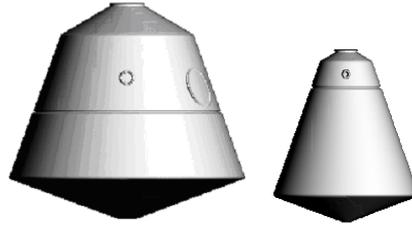
**Figure 4:** Illustration of the vehicle sent to Mars orbit. For the standard option, the vehicle is on the left and for the single habitat option, it is on the right. The separation between the command module and the service module is visible. The heat shield at the bottom protects the vehicle during Mars aerocapture. The heat shield of the command module for Earth atmosphere re-entry is hidden behind the service module.
