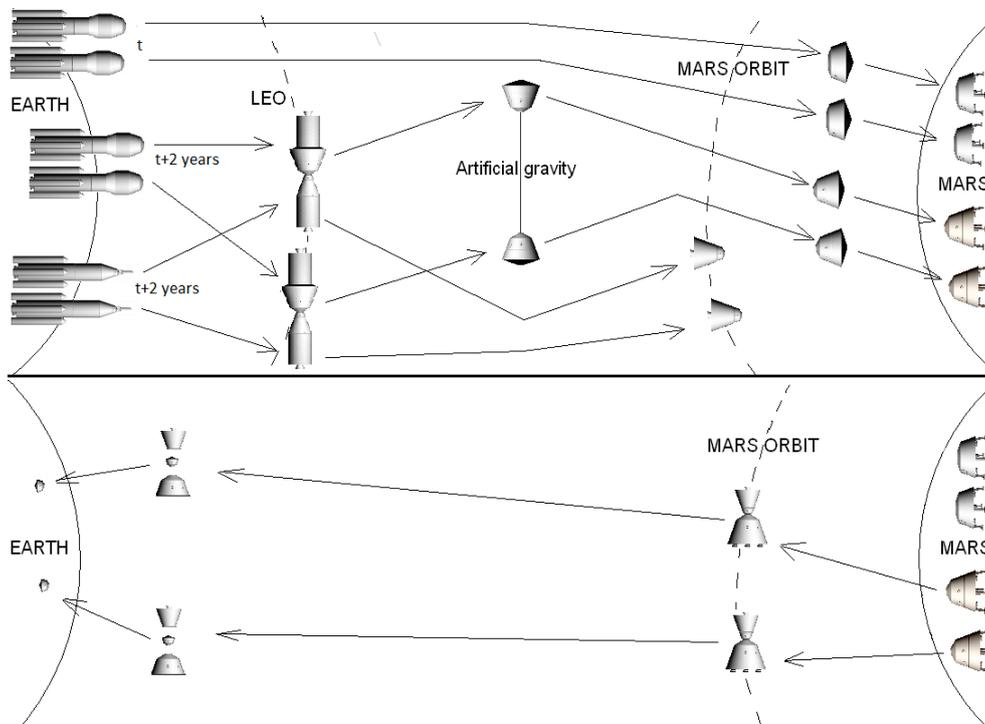
**Figure 3:** Single habitat option. The ERV sent to Mars orbit are smaller. Also, the habitat vehicles landed on Mars are the two Mars ascent vehicles. The Earth re-entry vehicles are small capsules.
