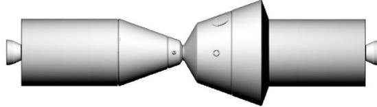
**Figure 6:** Junction in LEO between the ERV and the habitat lander. The astronauts are transferred to the main habitat while consumables for the return are transferred to the capsule. The TMI propulsion stage is still attached to the vehicles. At the end of the stay on Mars, the habitat lander will have to come back to Mars orbit and connect with the ERV in a similar way (without TMI propulsion stages).
