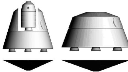
**Figure 5:** Illustration of the cargo landers. On the left, the payload of the standard option is mainly a light Mars ascent vehicle (dry). On the right for the single habitat option, there are only the ISRU and power systems but they are heavier in order to comply with the constraint of producing more propellant. In both cases, the shape is optimized for aerocapture and then entry descent and landing with a large heat shield located below the lander.
